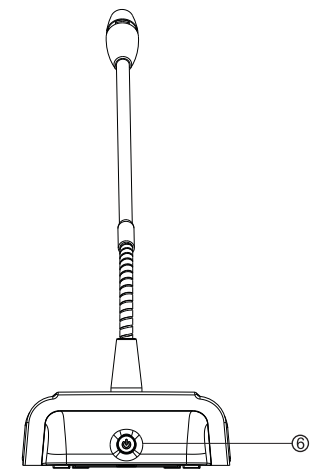
⑥ Battery switch (with indicator light): Press and hold the switch for 1.5 second to turn on the power of the unit. Press the power switch again for 3 seconds to turn off the unit.
